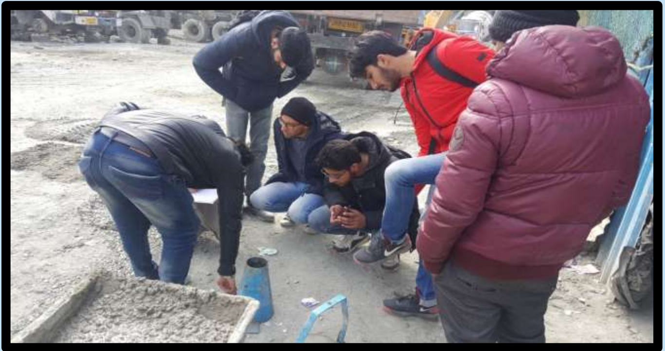
Students inspecting workability of concrete using slump test at a construction site at Mohali Punjab during their NITTTTR tour
